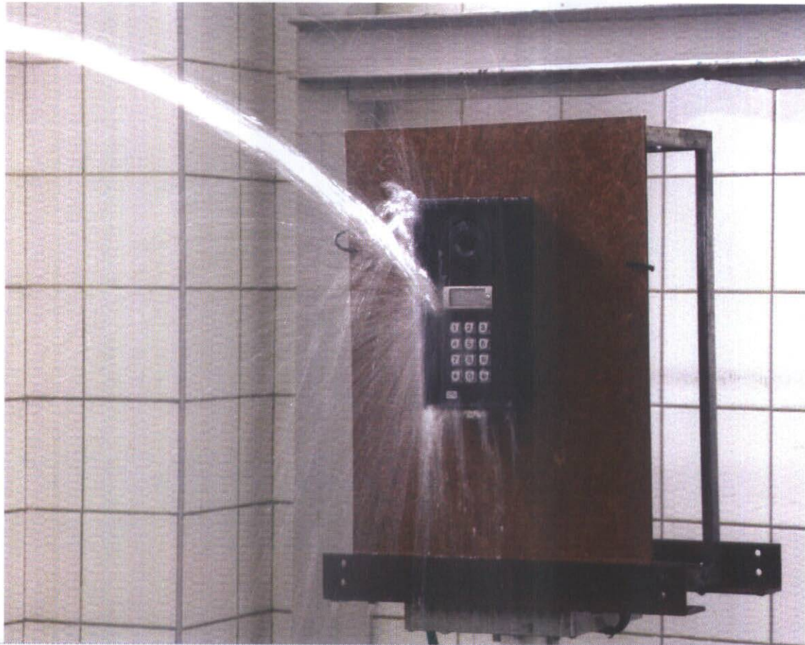
Fig. 10 - IP X5 testing of specimen 2N® Helios IP Force 9151101CK
