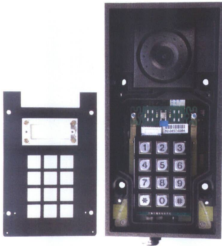
Fig. 13 - sealing of the specimen 2N® Helios IP Force 9151101CK
