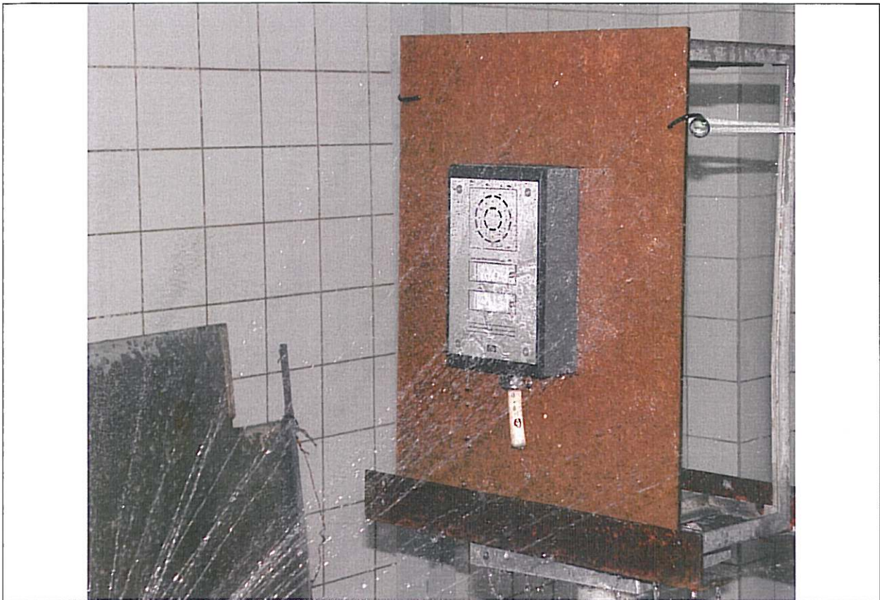
Fig. 3 - IP X4 testing
